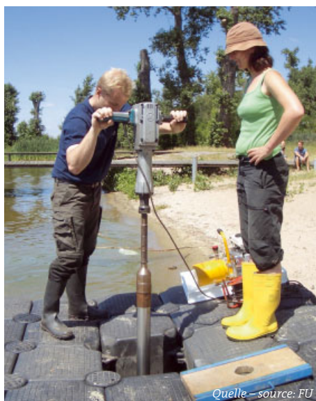
Sedimentkernentnahme am Wannsee zur Untersuchung der „Clogging“ Zone – Sediment coring at the shore of lake Wannsee to investigate the "Clogging" zone
