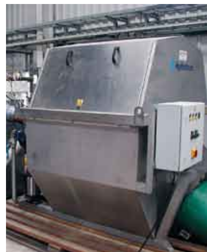
Mikrosiebanlage Microsieve pilot
