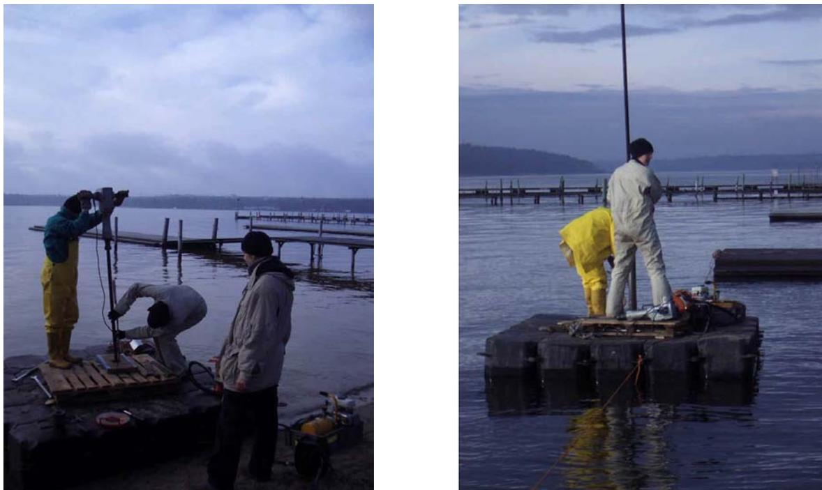
Figure 54: Taking cores from the clogging layer at Lake Wannsee in 1 m (left) and 40 m (right) distance from the shore.
